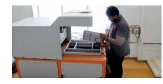
Plastic Shop is a place where students learn to turn plastic into permanent objects such as protective covers by identifying and acquainting with suitable materials. Students learn to design wood, machined aluminum molds, which are used to develop different shapes with the use of vacuum forming machines.
